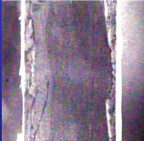
(c) Pitting corrosion
