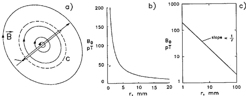
Figure 1. a) The magnetic field  $\vec{B}$  produced by a current  $I$  flowing in a long, straight wire. b) Linear and c) log-log plots of the strength of the magnetic field ( $B_\theta$ ) encircling a wire that is carrying a 1  $\mu\text{A}$  current.
