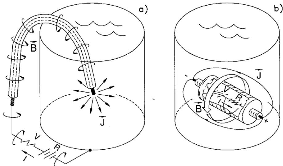
Figure 5. a) A point current source formed by the end of a wire immersed in a saline-filled metal bucket and connected to a battery. b) A self-contained current source consisting of two electrodes connected to a battery and a resistor, which are surrounded by a layer of insulation. The magnetic field, indicated by the broad arrow, encircles the source.
