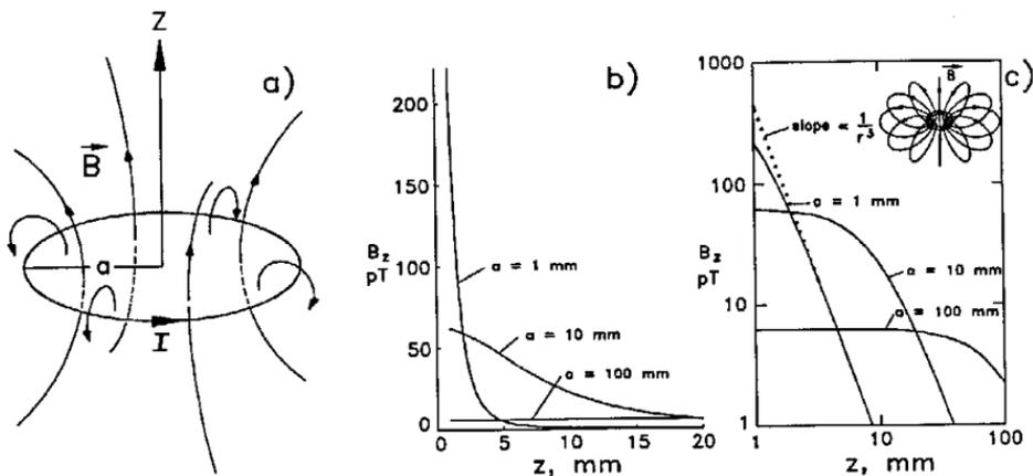
Figure 2. a) The magnetic field  $\vec{B}$  produced by a current  $I$  flowing in a loop of wire of radius  $a$ . b) Linear and c) log-log plots of the strength of the magnetic field  $B_z$  along the axis of the loop, which is carrying a  $1 \mu\text{A}$  current, for loops of three different radii. The inset in c) shows the dipolar magnetic field of a small current loop.
