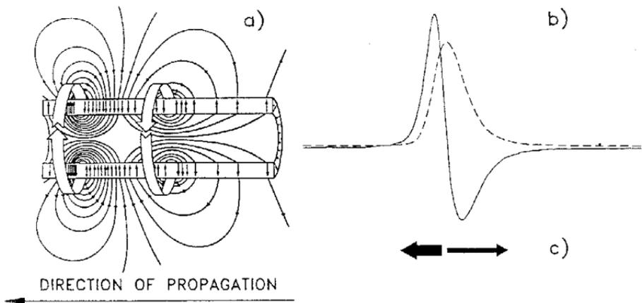
Figure 9. a) The electric current (thin arrows) and magnetic field (wide arrows) associated with a propagating nerve action potential. The thickness of the membrane is greatly exaggerated. b) The corresponding transmembrane potential (dashed) and the axial, intracellular action currents (solid). c) The depolarization (D) and repolarization (R) current dipoles consistent with a) and b).
