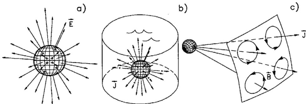
Figure 4. a) The electric field  $\vec{E}$  produced by a positively-charged sphere in air. b) The electric current density  $\vec{J}$  produced when the sphere in a) is immersed in saline to form a point current source. c) An illustration of how the magnetic fields  $\vec{B}$  from the lines of current in b) cancel each other so that a point current source produces no magnetic field.
