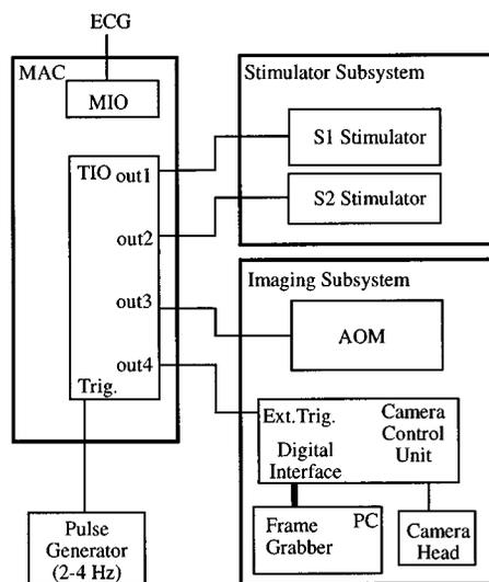
FIG. 2. Block diagram of the synchronous imaging system.
