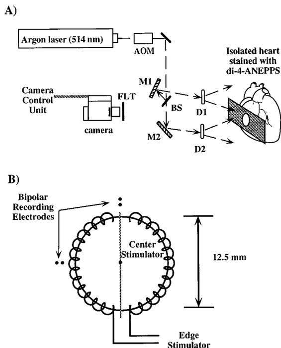
FIG. 1. (A) Schematic drawing of imaging setup. (B) The imaging window.
