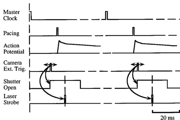
FIG. 3. Timing diagram of the system. Note that the “shutter open” and “laser strobe” signals are locked to “camera external trigger” with fixed delays.
